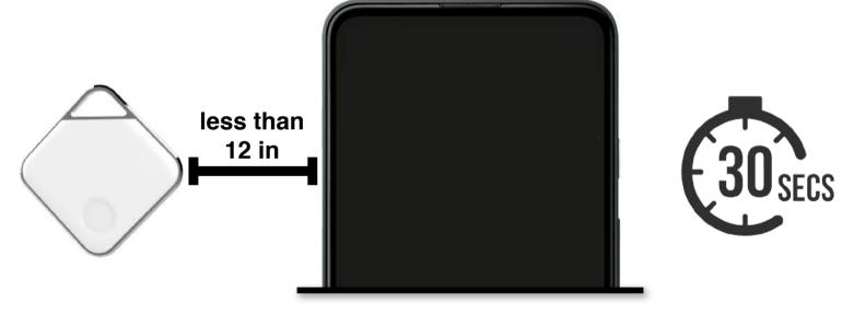
This 30 seconds will ensure pairing is fully established. The phone's Bluetooth must remain turned on for the PRD to function properly.
