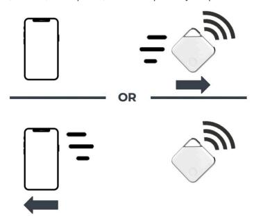
The PRD can be put into "Selecting Home or Travel" mode by quickly pressing the button five (5) times and then holding the button down until a single beep or double © 2021-2025 Prox Devices, Inc. All rights reserved.
