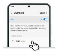
4. On the **Bluetooth pairing request** pop-up, select **Pair**. A solid blue light on the PRD and a connection sound will confirm a successful pairing.
