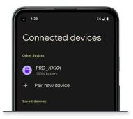
If pairing is done in the Bluetooth section, you will need to go back to **Connected devices** to see that the PRD is paired with the phone.
