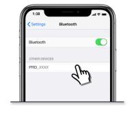
3. On the **Bluetooth Pairing Request** pop-up, select **Pair**. A solid blue light on the PRD and a connection sound will confirm a successful pairing.
